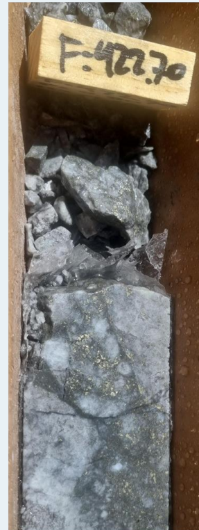
Visible copper and zinc sulphide mineralization from DDH-PO-01, 413m below surface.
