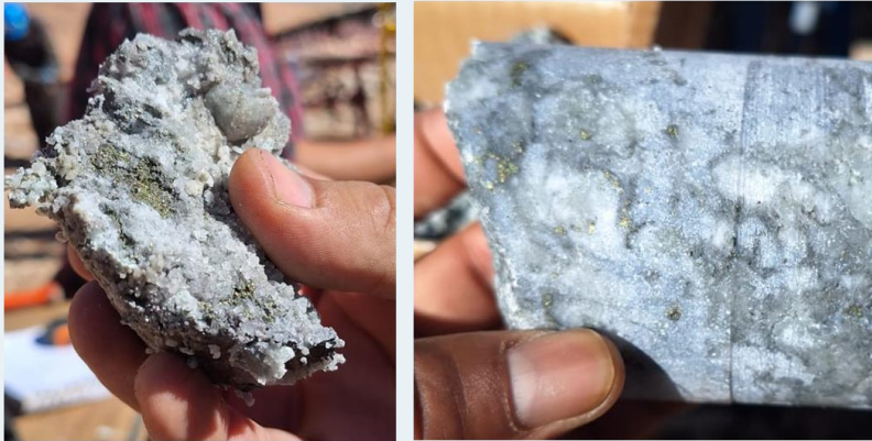
Drillhole DDH-PO-01. Sphalerite mineralization
