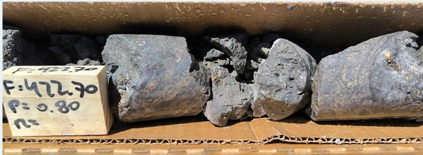
Visible copper and zinc sulphide mineralization from DDH-PO-01, 413m below surface.
